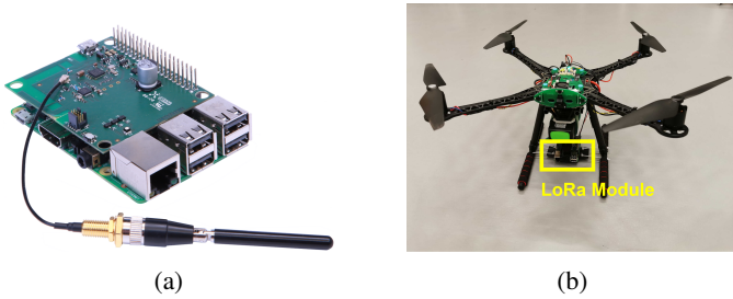
Fig. 3: (a) LoRa 2.4 GHz module stacked on a Raspberry Pi 4. The optional external antenna shown was not used in the experiments. (b) The UAV carrying the LoRa module.
