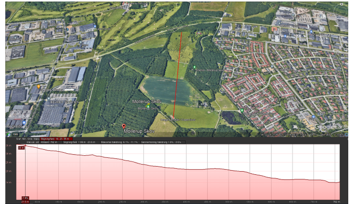
Fig. 2: Aerial photo of the test site (top) with a contour line for the example of an 800 m LOS experiment (bottom).
